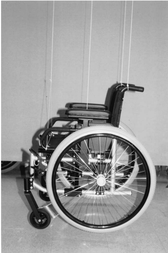
Fig. 1. Set-up for the determination of wheelchair moment of inertia. Strings located on the push handles and front seat of the wheelchair are equidistant from the wheelchair COM that is illustrated by the plumb bob.
