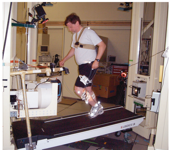
Fig 1. A subject is shown running downhill on a treadmill in the High-Speed Biplane Radiographic System. Images were acquired simultaneously at 250 frames/s for the two views (60° separation).
