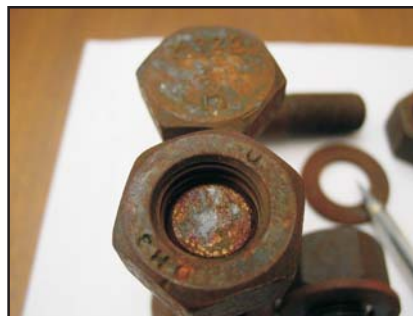
Figure 3: The rust increases the turning force (torque) needed by causing more friction or resistance between the threads.
