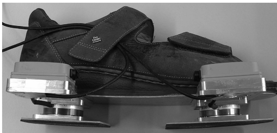
Fig. 1. Picture of the instrumented shoe with force/moment sensors beneath the heel and forefoot and inertial sensors rigidly attached to the force/moment sensors. A thin flexible glass-fiber plate connects both sensors allowing regular flexion of the foot during push-off.
