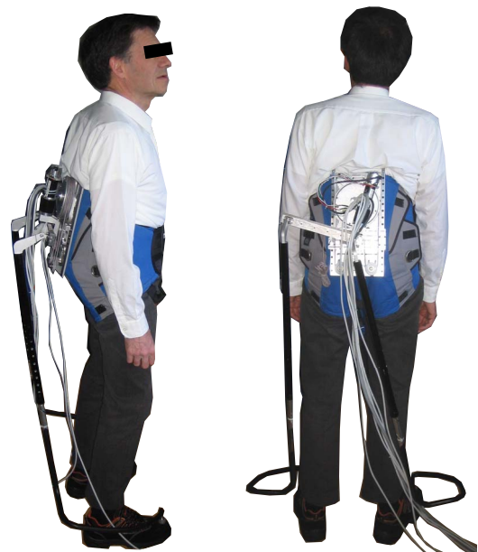
Fig. 1. Pictures of MoonWalker, a lower-limb exoskeleton able to sustain part of user’s weight based on passive gravity compensation
