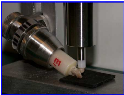
Fig. 1. Fall configuration designed to test the proximal femur subject to failure.
