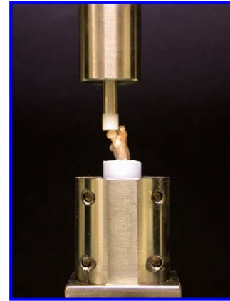
Fig. 2. The axial compression parallel to the femoral shaft vertical axis for testing the proximal femoral strength.
