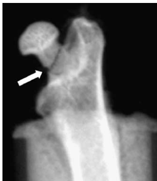
Fig. 4. Representative fracture mode from 'fall-configuration test'. White arrow: the fracture line.
