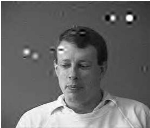
Figure 4.12: 3-D subband PVQ coding video sequences at PSNR=32.2 dB, 0.6 bpp, recovered from average shadowed mobile satellite channel during deep fading, channel SNR=10.5 dB, BER= 10^{-3}
