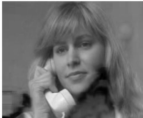
Figure 3.15: Transmitted video through average shadowed mobile satellite channel, channel SNR=10.0dB, RS & TCM coding, one of 200 error frames in a total 15000 video frames
