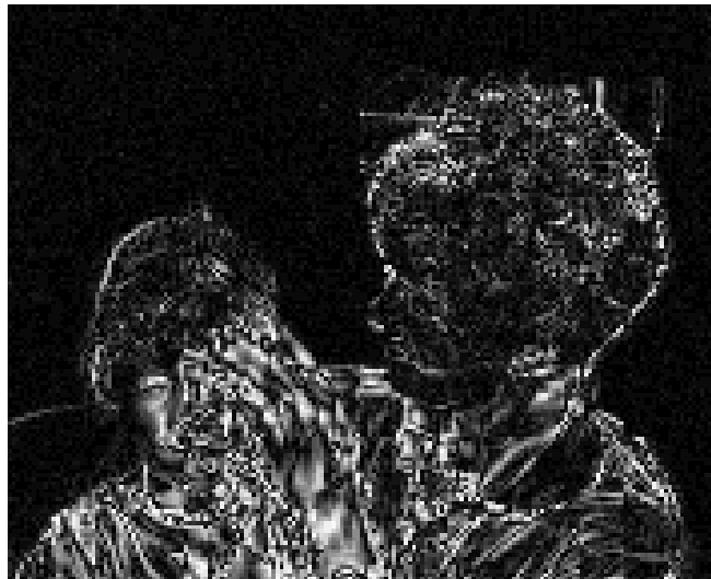
a) Mother-Daughter, Frame 16 Error Image - Quadtree-MDL 15 kb/s, PSNR = 31.59 dB
